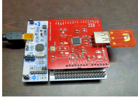
Figure 3.6: First PCB for testing minimal circuit for AD5941
